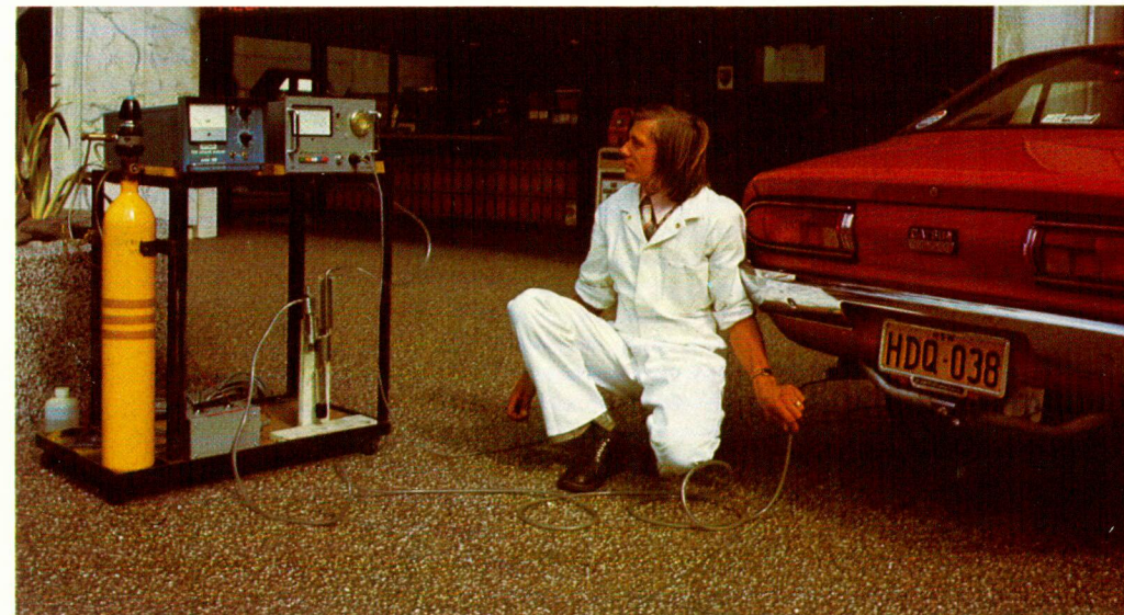
Checking an exhaust for carbon monoxide emission.
