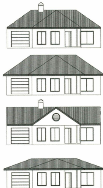
FIGURE 62. ROOF FORM HAS A SIGNIFICANT IMPACT ON THE LOOK OF THE HOUSE
