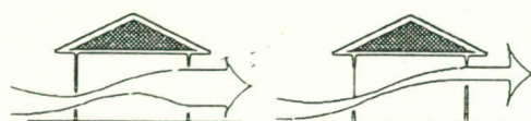
Small, low opening on the windward side and large high openings on the down-wind side for good cross-ventilation.
