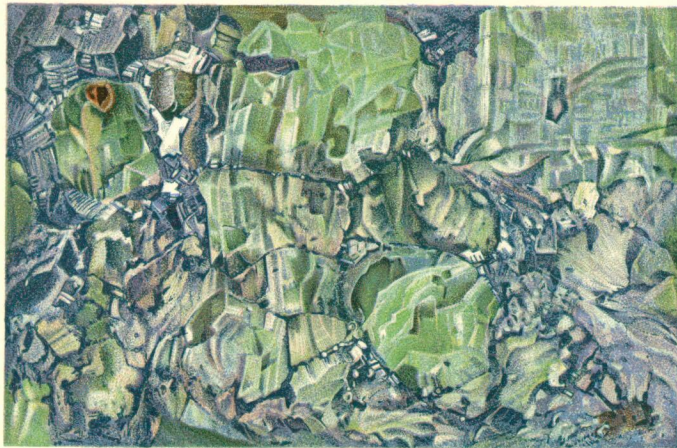
Pegmatite with green felspar, replaced in part by galena; zinblende, garnet, and quartz.
