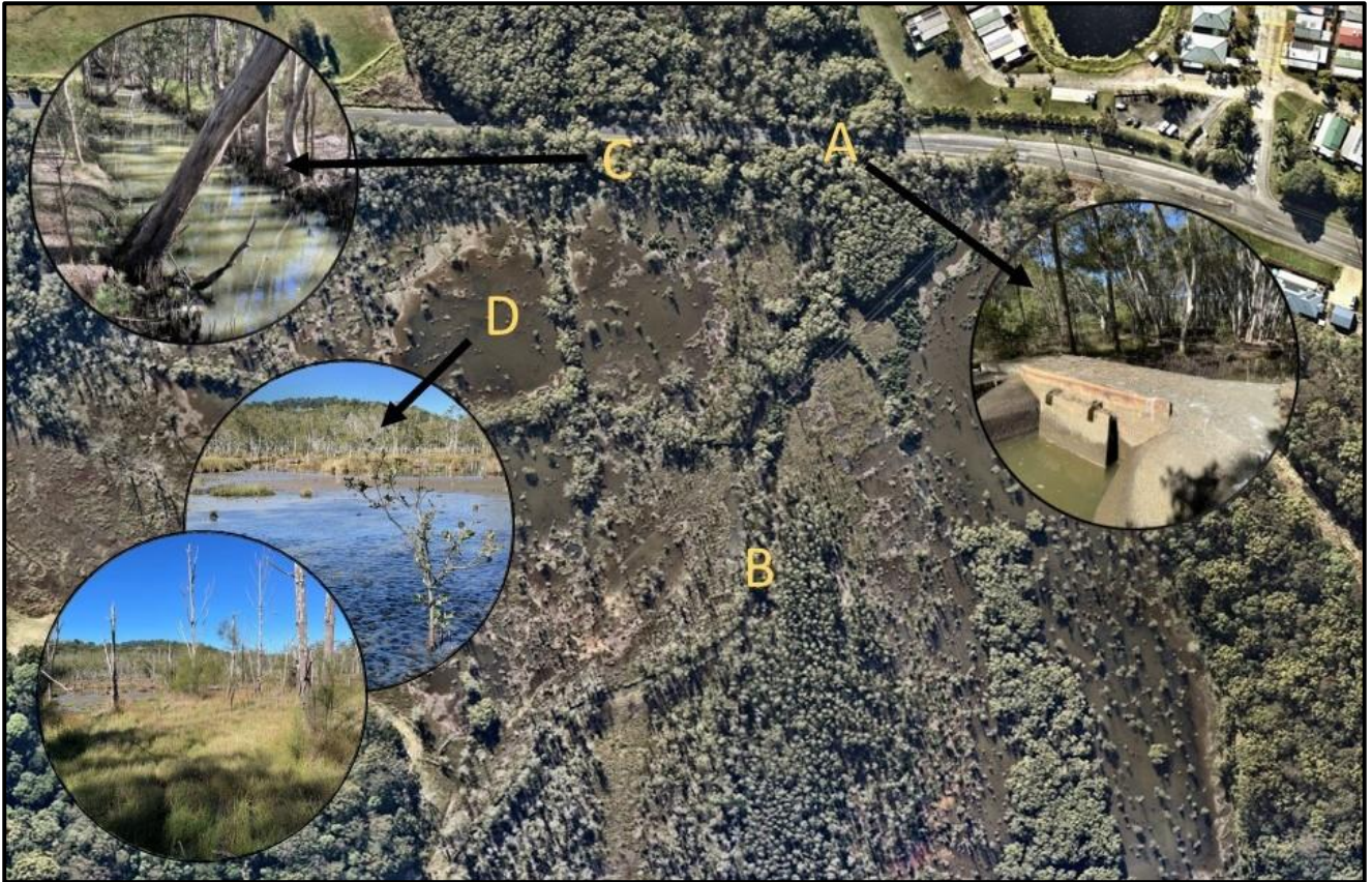
Figure 15 Site to the south of Piggabeen Road. A, legacy flood gated culvert. B, natural creek line. C, drain parallel to the road. D, impact of saltwater incursion into previously freshwater habitats. Images: Nearmap (base).
