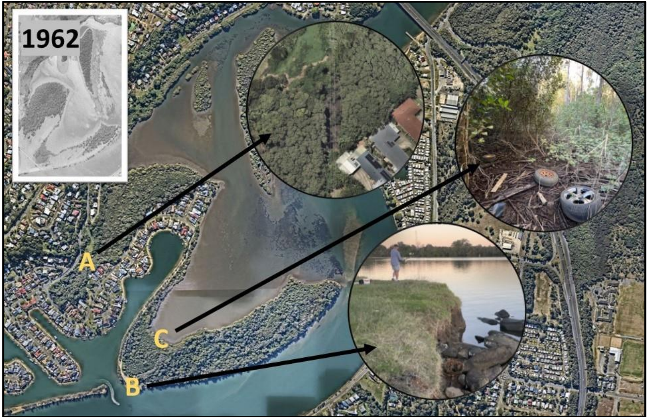
Figure 53 Chinderah Bay including changes to morphology over time. A, powerlines crossing the wetland were installed using a levee that continues to impede tidal flows. B, erosion and failed bank armoring. C, active sediment accretion with debris. Images: Nearmap (base) and NSW Government Spatial Services (inset).
