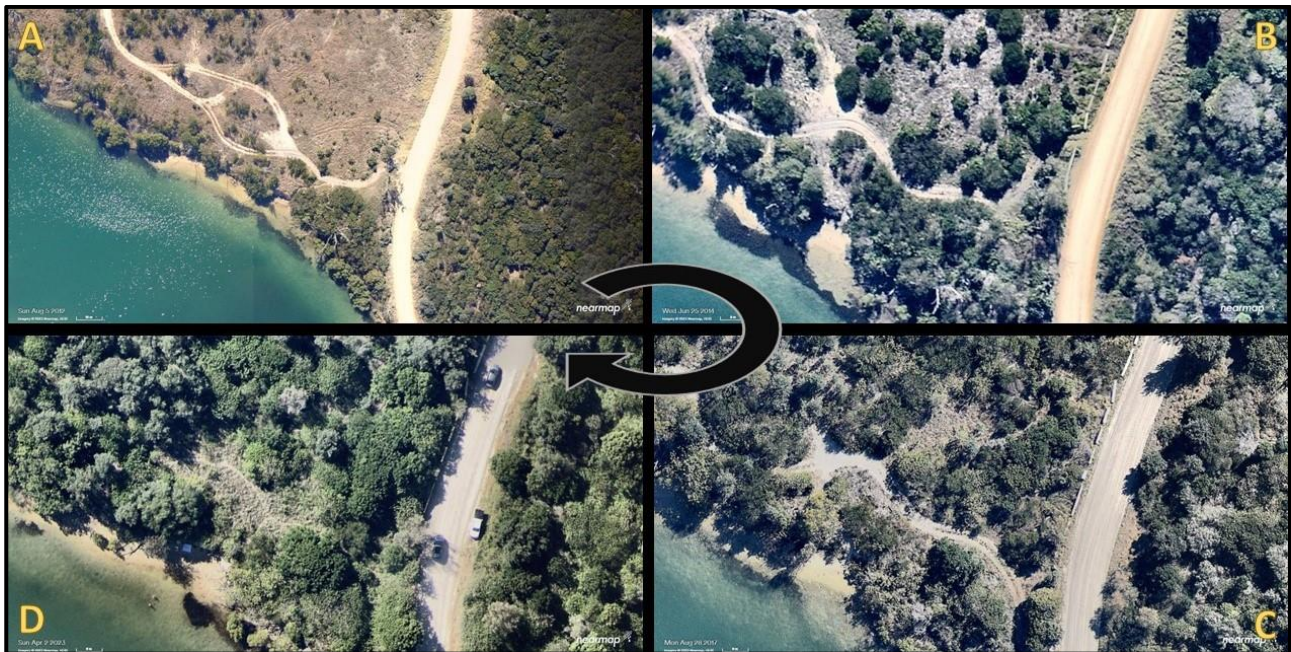
Figure 43 Restricting vehicular access to Kerosene Inlet. A, extensive vehicular damage to saltmarsh and mangrove habitats in 2012. B, avoidance of installed bollards in 2014. C, access point shifted after bollard reinforcement in 2017. D, pedestrian access only in 2023 with substantial recovery of intertidal and terrestrial vegetation. Images: Nearmap.
