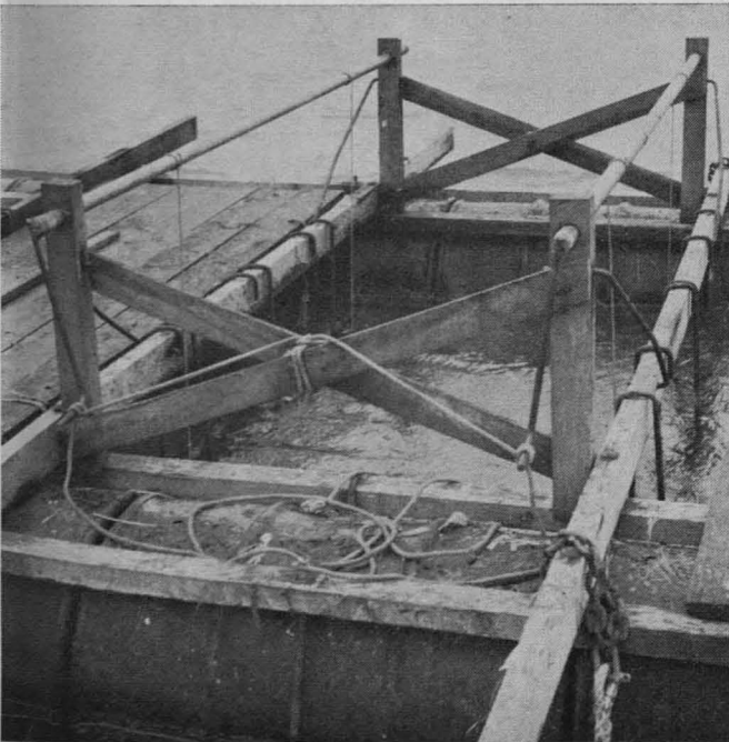
FIGURE SEVEN: Moveable winch, to lift cage with trays. (Photo Lindemann.)
