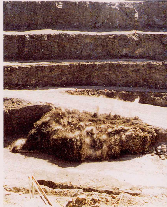
Good blast design results in a predicted size construction material product ready for further processing
