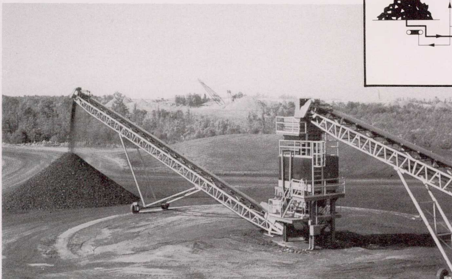
Left: An Illinois Basin Coal Producer uses the GAMMA-METRICS Analyzer to sort raw coal according to sulphur content.
