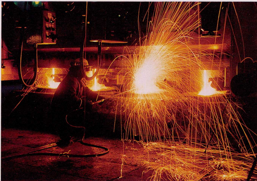
Steel blending in an electric arc furnace at the BHP mini steel mill
