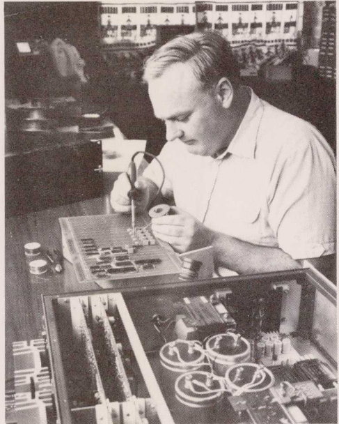
David Dagg, Technical Officer of the Geophysics Section, designed and constructed all instrumentation for the project. He is seen here constructing the digital receiver module
