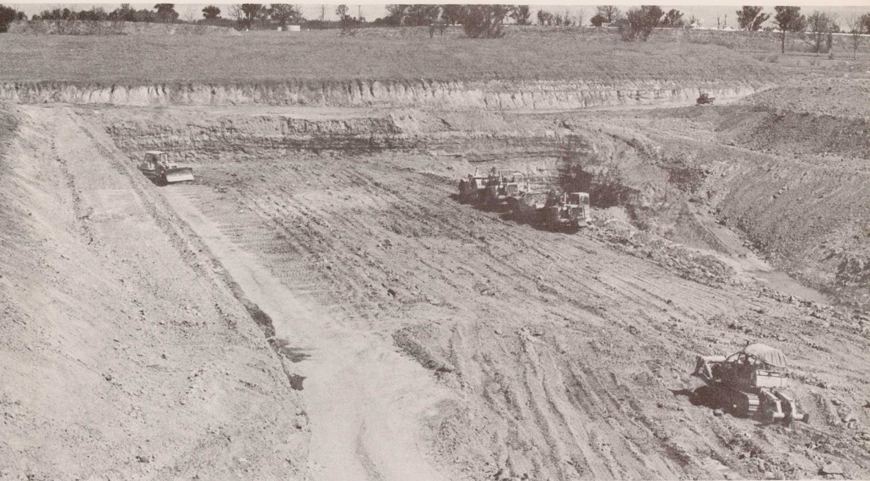
Selective extraction of clay/shale in the Bringelly Shale at Badgerys Creek (Boral Bricks (N.S.W.) Pty Ltd)
