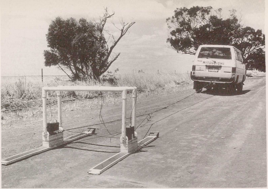
Ground penetrating radar unit in a sled configuration for towing by a vehicle (courtesy of Paul Baker, Monash University)
