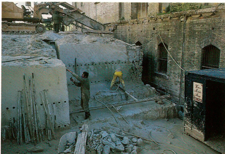
Quarrying for yellowblock compatible sandstone in Kent Street, Sydney, adjacent to the historic Grafton Wharf quarry, on the site of the present Maritime Services building
