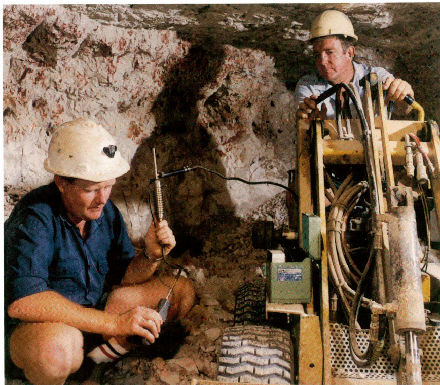
Underground testing of diesel exhaust gases in an opal mine
