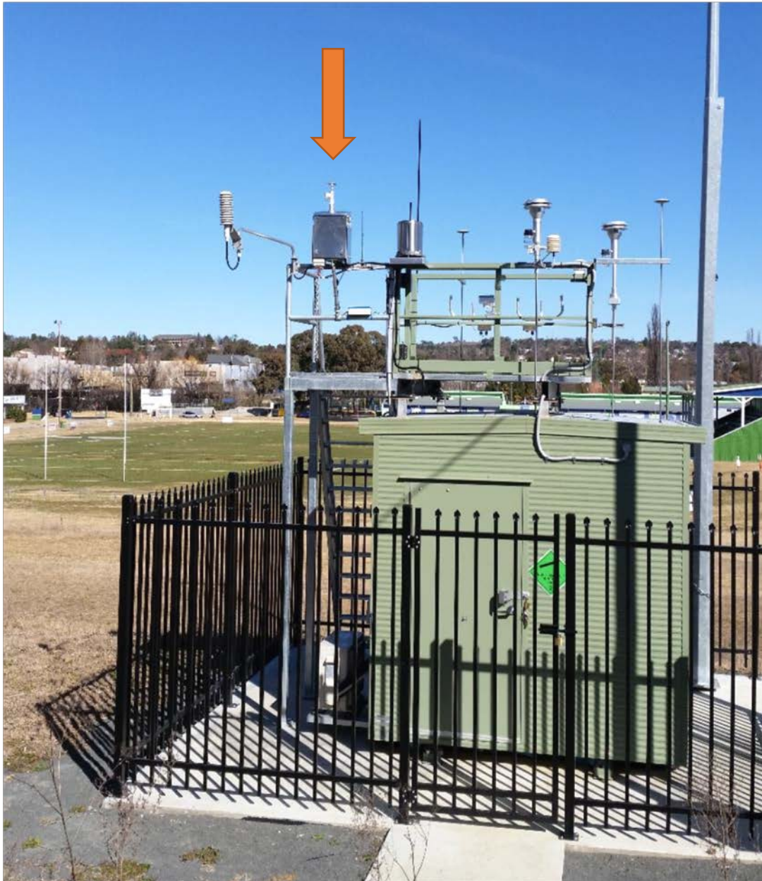
Photo 1: Armidale Air Quality monitoring site with added DustWatch equipment (below arrow). Photo: Stephan Heidenreich
