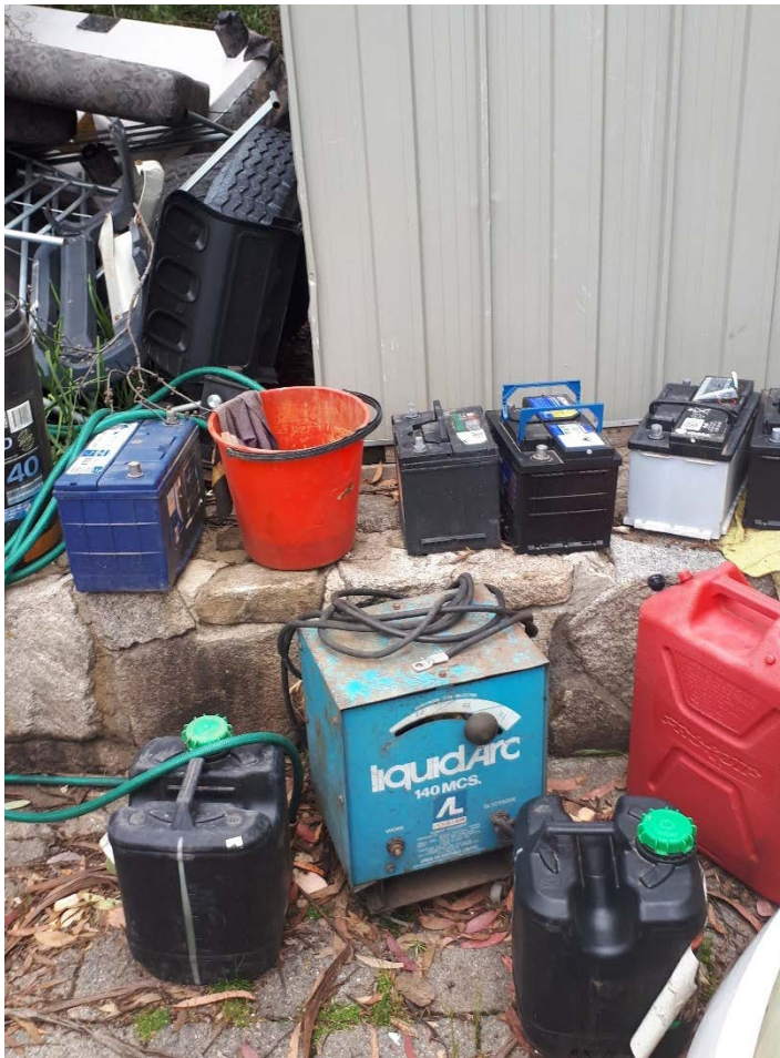
Figure 4 Incorrect storage of lead batteries and petroleum products. Photo: P McCarthy/DPIE
