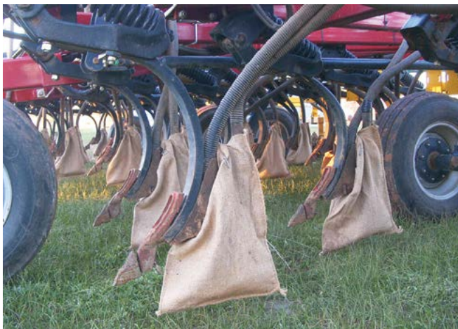
A hessian bag can be tied to each tyne to collect product during seeder calibration.
