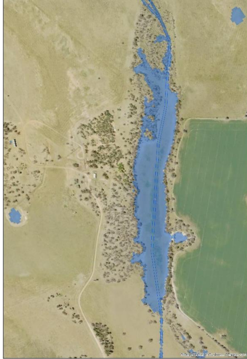
Figure 3. This inundation map was produced using the multi-index method from an image captured on 6 June 2022. A comparison is shown against a drone image taken on the 7 June 2022 (Figure 4) during field work for the Floodplain Pools Fauna project (see EOMRP Theme 4). The inundation mapping closely represents what was observed in the field.
